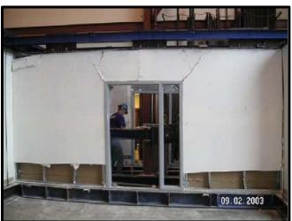
**Step #6:** Stiffen the building (longer walls, more coupling, etc.). Reduces the maximum drifts from around 1.4% to 1.0%.
